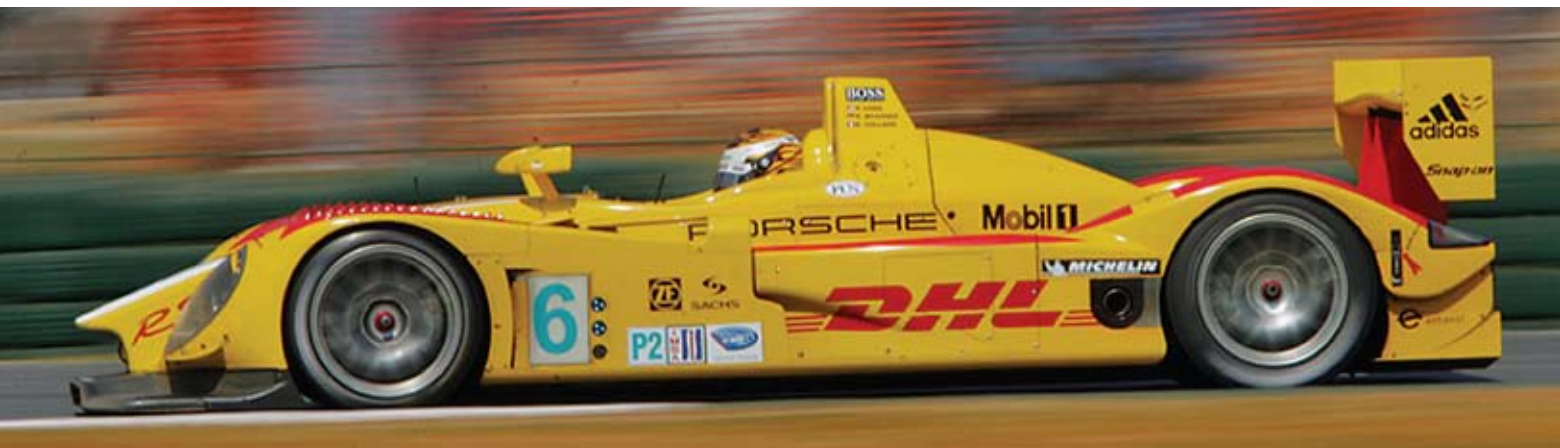
The initial Green Challenge trophy for the ALMS LMP2 (prototype) class at the 2008 Petit Le Mans race went to a E10 gasoline direct-injected, 503-hp (375-kW) Porsche RS Spyder prepared by the Penske Racing team.
