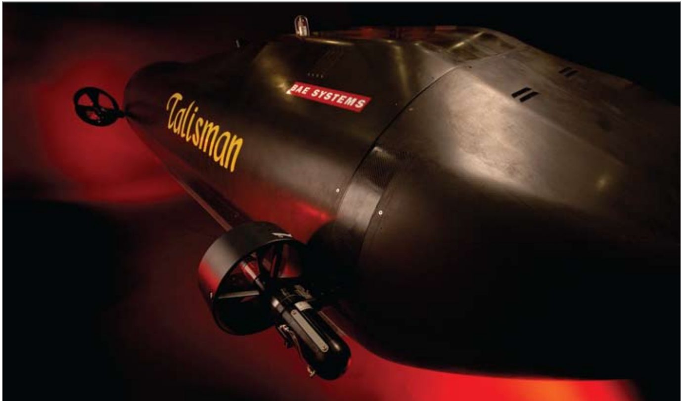
BAE Systems' Talisman UUV: the composite hull structure was developed by Lola, the racing car designers [BAE Systems and Lola Cars]
