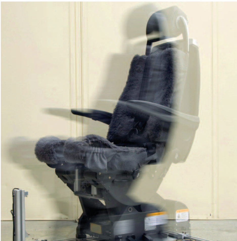
The Boeing 787 Dreamliner's crew seat undergoing vibration testing at MIRA.
